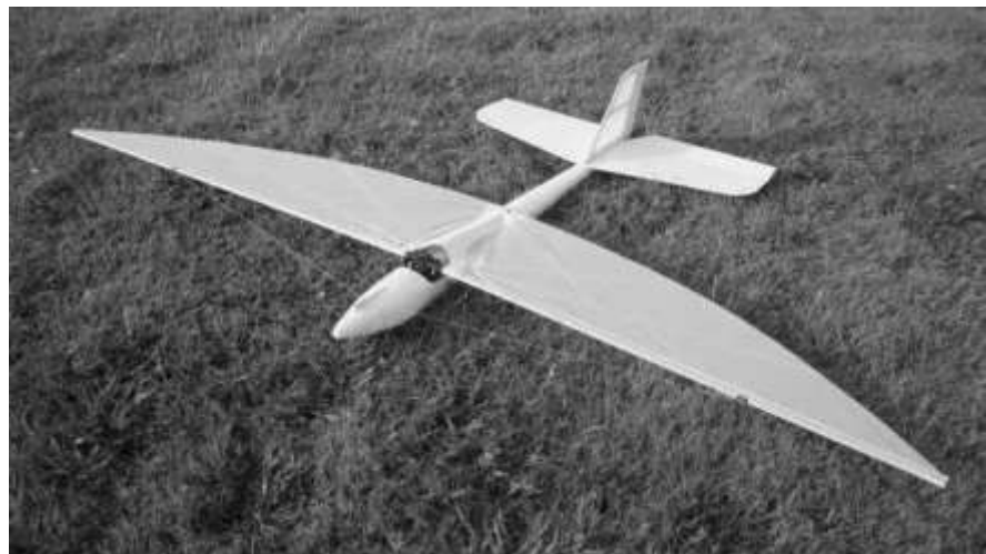
Crossbow achieves efficiency with cord-tensioned wings and sailplane-like body.
