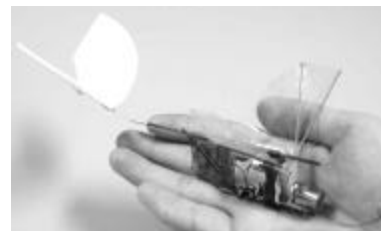
Figure 14: Battery-powered ornithopter MAV
